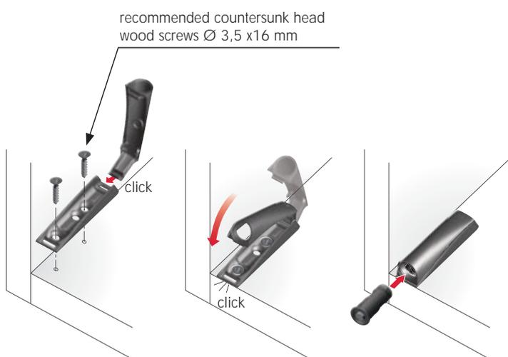
recommended countersunk head wood screws  $\varnothing$  3,5 x16 mm
