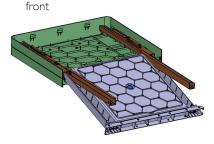
Position drilling template on the tabletop and define the wanted positions.
