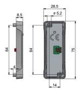
RFID reader L033-A02 with optional spacer
