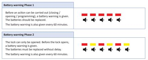
The settings are saved even without a power supply (e.g. in case of battery replacement, or in case the batteries should be completely empty). Battery replacement should be carried out within 5 minutes.
