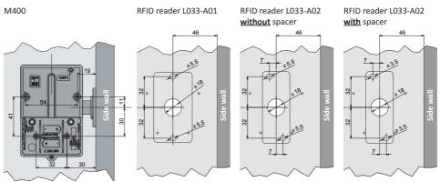
CAUTION: - For mounting the RFID reader L033-A02 • without spacer please use drill holes of 5,5mm. • with spacer please use drill holes of 3,5mm.
