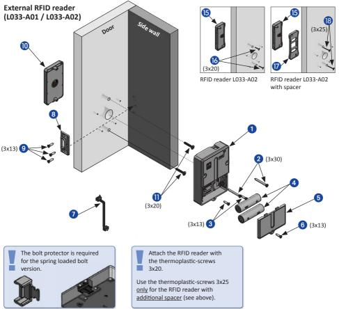
Please note the different mounting positions and drilling pattern for the RFID readers.
