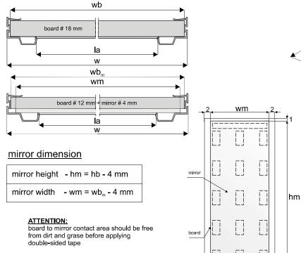
Broken line indicates recommended positioning of double-sided tape
